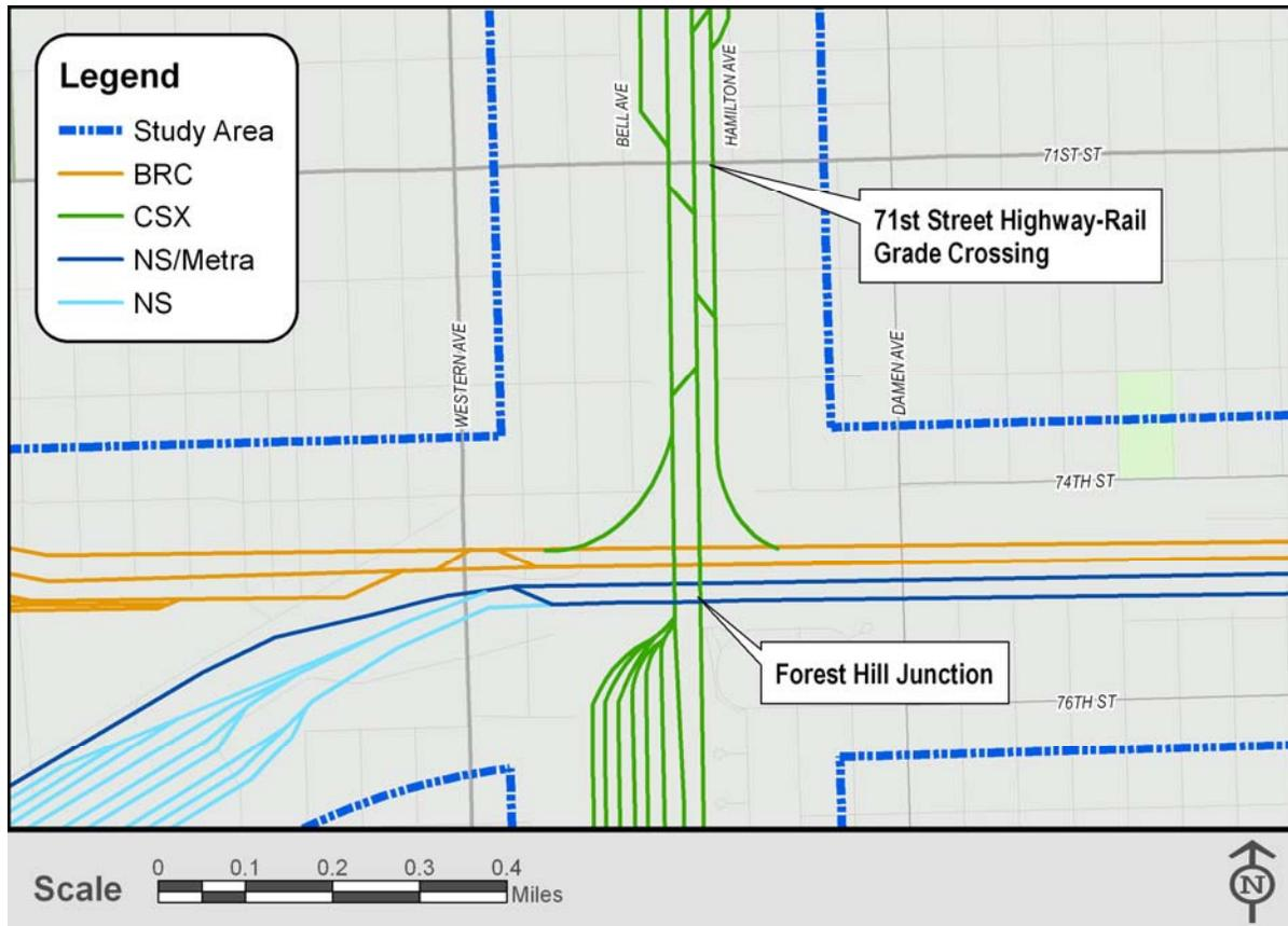
Figure 2-4: Existing Track Schematic – Forest Hill Junction
