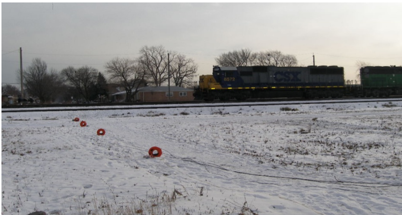
Figure 3.7-11: Ground Vibration Measurements along the CSX north of Forest Hill Junction
