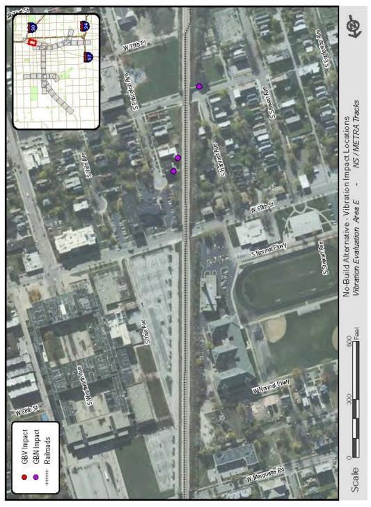
Figure 5-43: Locations Where No-Build Alternative Vibration Exceeds FTA Threshold
