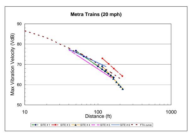
Figure 3-1: Ground-Borne Vibration from Metra Trains at 20 mph
