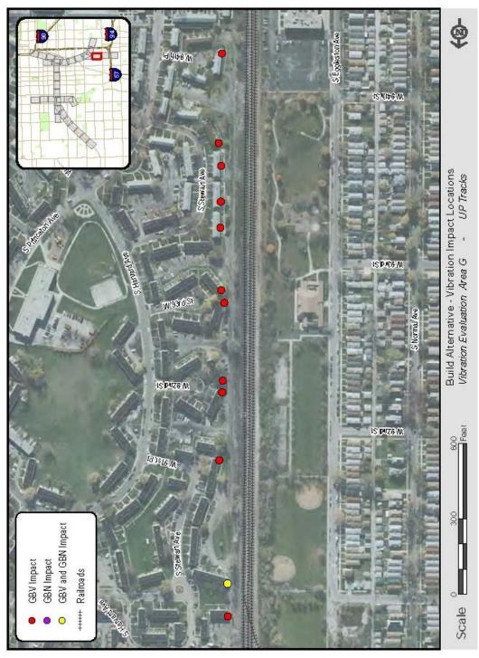
Figure 5-34: Build Alternative Vibration Impact Locations
