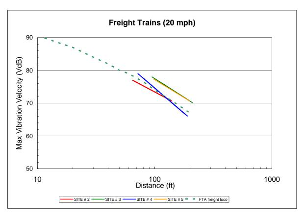
Figure 3-3: Ground-Borne Vibration from Freight Trains at 20 mph
