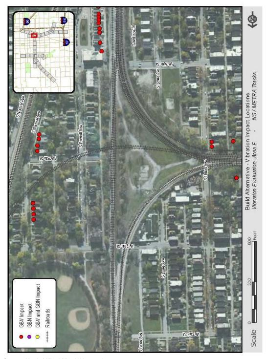
Figure 5-26: Build Alternative Vibration Impact Locations
