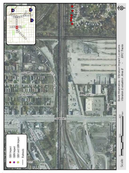
Figure 5-10: Build Alternative Vibration Impact Locations
