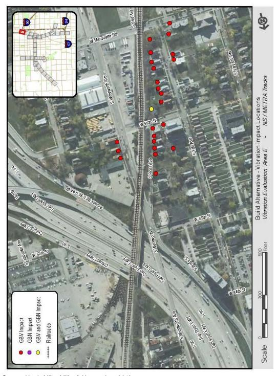
Figure 5-21: Build Alternative Vibration Impact Locations
