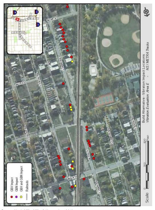
Figure 5-23: Build Alternative Vibration Impact Locations
